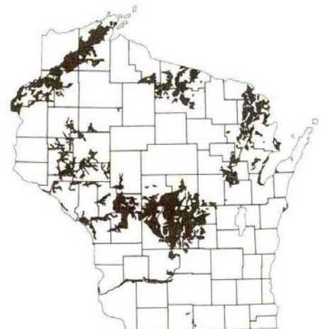
Figure 2-24. Sandy surficial soil horizons commonly total more than 36 inches in thickness and are underlain by acid sand glacial outwash.
